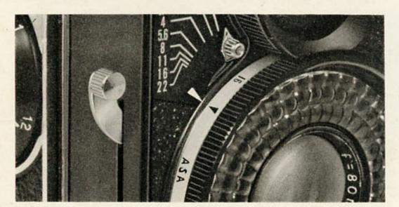
Set the red triangle on the ASA Film Speed Control Ring in line with the red triangle on the manual control plate.
