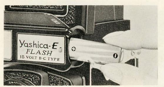
Slide in the 15volt dry battery with the plus(+)facing in. (Follow the diagram in the chamber.) Replacement batteries are available at your camera store or any electronics supply house. Ask for NEDA 220 type or equivalent.
